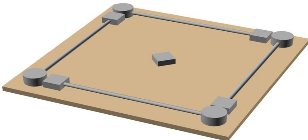
**Figure 1.** Functional outline of a device for precise positioning of agricultural machines with folded arms for mounting MEMS and GPS sensors. In the center of the device there is a central sensor that allows to increase the precision of the measurements.
